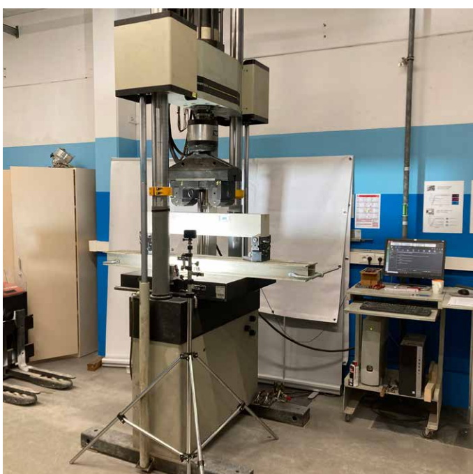
Figure 1: Test setup four-point bending tests
